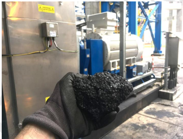
Figure 4 Coke after Crusher with ECHO
